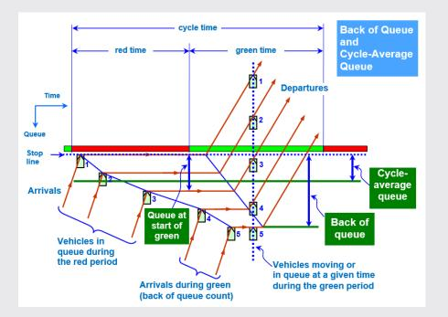
Back of Queue is important for modelling of short lane overflow and queue spillback in networks
