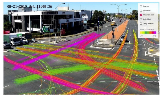
Fig. 3. Computer Vision-based automated conflict data extraction method.
