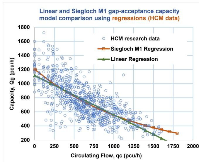
**Figure 4 - Comparison of linear model and the Siegloch M1 exponential capacity models using HCM roundabout capacity research data**
