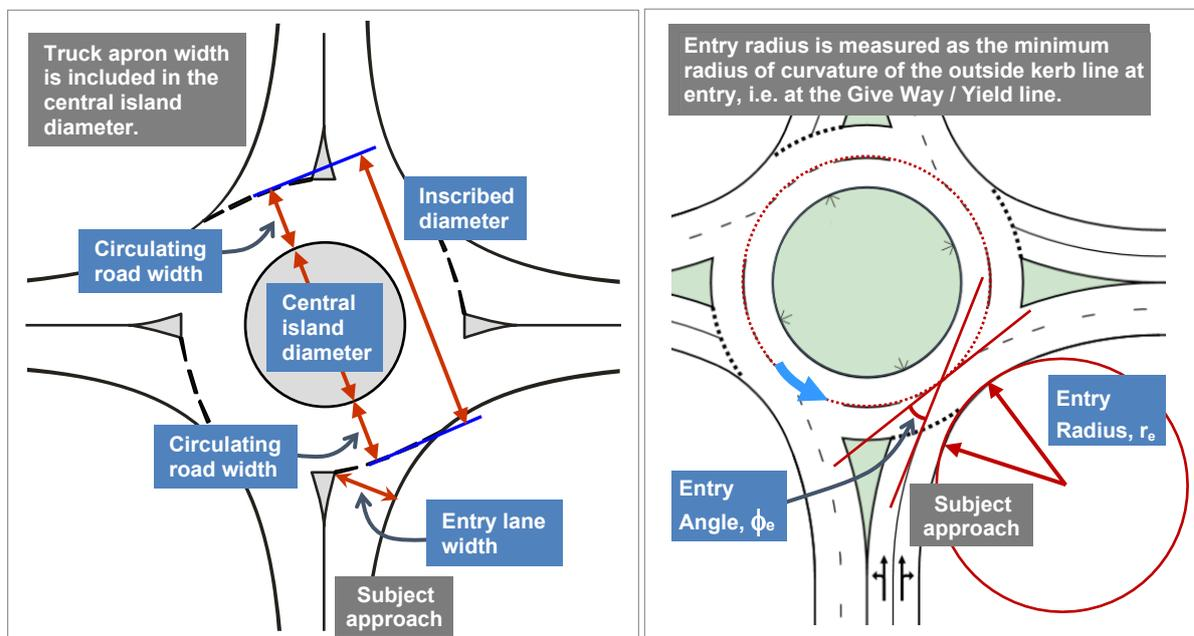
Figure 10 - Inscribed diameter, entry radius and entry angle measurements in SIDRA INTERSECTION
