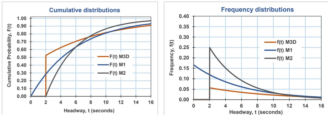
Figure 1 - Cumulative distributions and frequency distributions for M1, M2 and M3D (exponential) headway distribution functions
