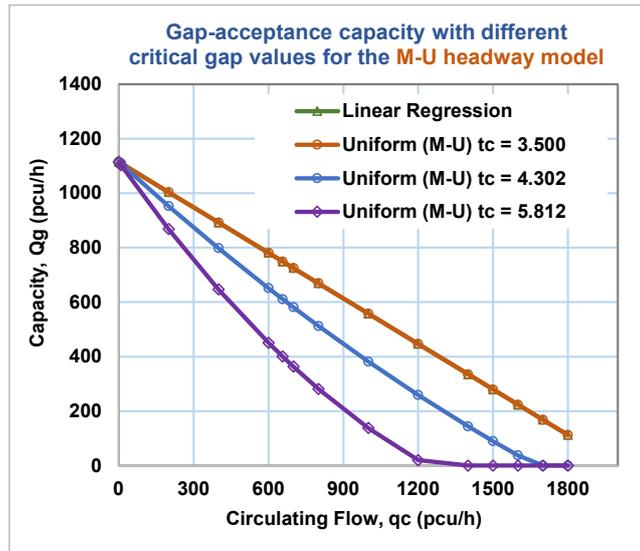
Figure 8 - Comparison of the gap-acceptance capacity model based on the uniform headway distribution (M-U) with a basic Linear model from regression using the HCM roundabout capacity research data using different critical gap,  $t_c$  values
