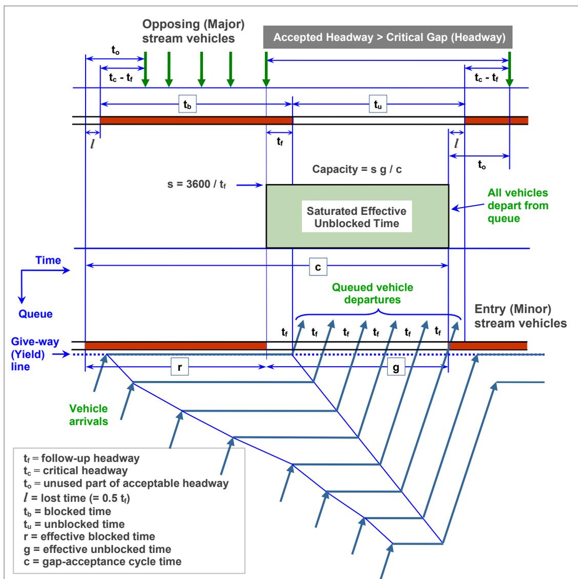
Figure 2 - Gap-acceptance capacity signal analogy concept
