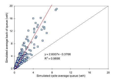
Figure 5 - Simulated cycle-average queue values vs average back of queue values for roundabouts
