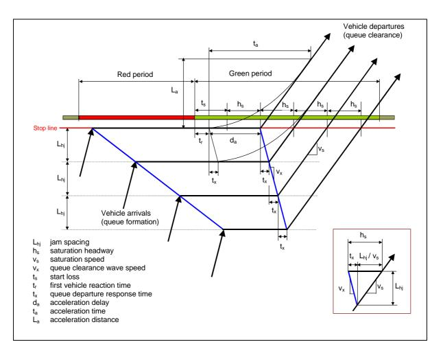
Figure 3 - The relationship between saturation headway, saturation speed, jam spacing, queue departure response time and queue departure wave speed
