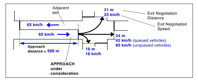
Figure A.4 - Definition of approach and intersection negotiation distances and speeds
