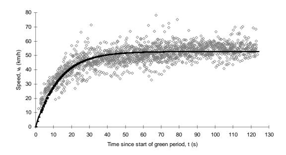
Figure 1 - Queue discharge speeds observed at the intersection of General Holmes Drive and Bestic Street in Sydney (through lane)<sup>14</sup>
