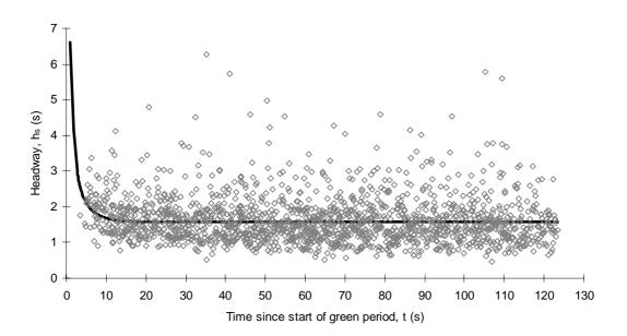
Figure 2 - Queue discharge headways observed at the intersection of General Holmes Drive and Bestic Street in Sydney (through lane)<sup>14</sup>
