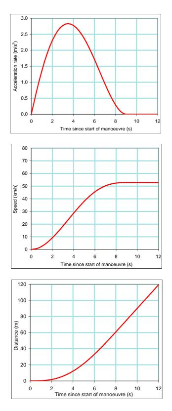
Figure 4 - Acceleration rate, speed and distance profiles for queue discharge manoeuvres determined for the site shown in Figures 1 and 2
