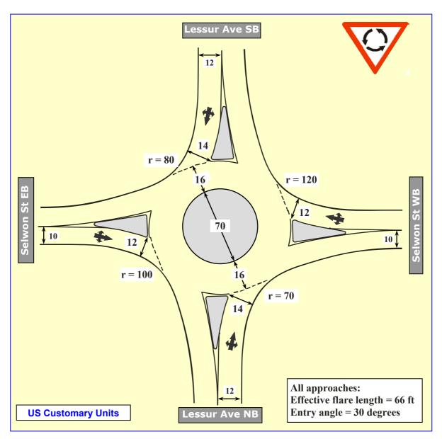
Figure 1 - Case Study - Single-Lane Roundabout, USA: Roundabout geometry
