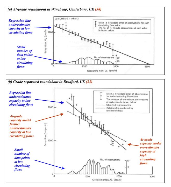
Figure 5 - Data from roundabout capacity surveys at UK roundabouts
