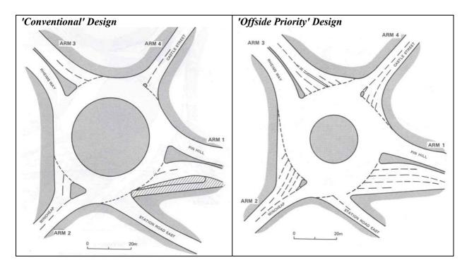
Figure 6 - Examples of 'Conventional' and 'Offside Priority' roundabout designs used in capacity measurements for TRL (UK) linear regression model (38)
