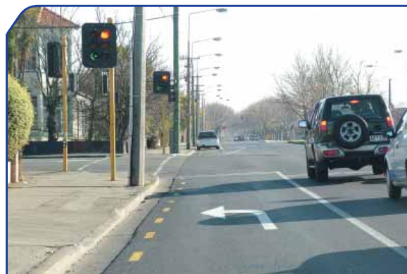
Figure 19 : No safe and legal waiting position for straight-through cyclists during left turn only phase.
