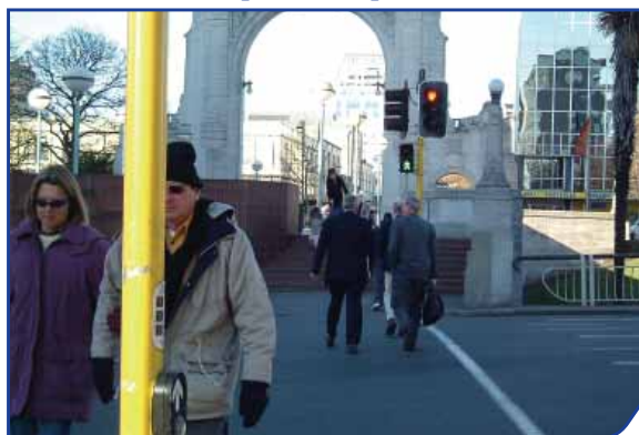
Figure 16 : A late start of the vehicle phase provides pedestrian protection at this T intersection.
