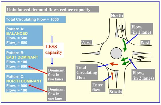
Figure 4.2 - The effect of the Origin-Destination (O-D) pattern on capacity
