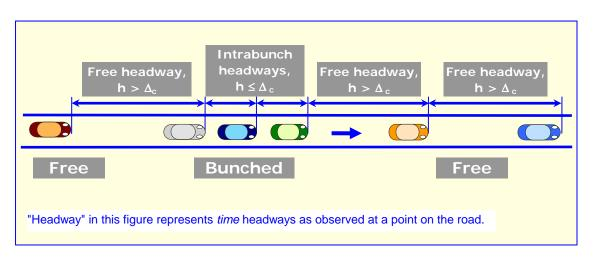
Figure 6.1 - Circulating stream parameters used in the bunched exponential model for estimating circulating stream headway distribution
