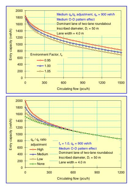
Figure 8.1 - Effect of the Environment Factor and the Adjustment Level for Arrival Flow / Circulation Flow Ratio for the dominant lane of a two-lane roundabout (inscribed diameter = 50 m, average lane width = 4.0 m, Medium O-D pattern effect, entry flow rate = 900 veh/h, no heavy vehicles)
