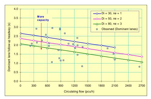
Figure 5.1 - Unadjusted dominant lane follow-up headway ( $\beta_{d1}$ ) as a function of the circulating flow for three roundabout cases: 1-lane roundabout with  $D_i = 30 \text{ m}$ , 2-lane roundabout with  $D_i = 50 \text{ m}$  and 3-lane roundabout with  $D_i = 80 \text{ m}$  (lane width = 4.0 m)
