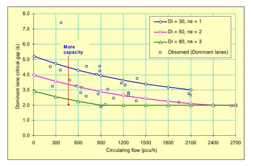
Figure 5.2 - Dominant lane critical gap corresponding to the unadjusted dominant lane follow-up headway as a function of the circulating flow for three roundabout cases: 1-lane roundabout with  $D_i = 30$  m, 2-lane roundabout with  $D_i = 50$  m and 3-lane roundabout with  $D_i = 80$  m (average entry lane width = 4.0 m)
