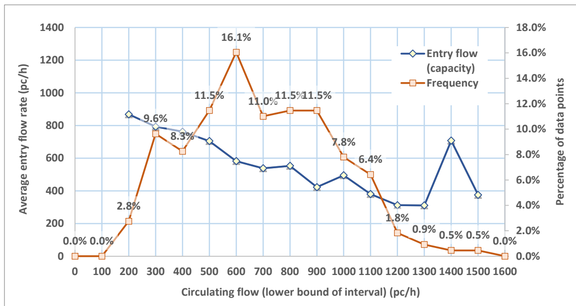
Figure 6.1 - Frequency of capacity data points as a function of the circulating flow and average entering flow (capacity) data in 100 pcu/h intervals
