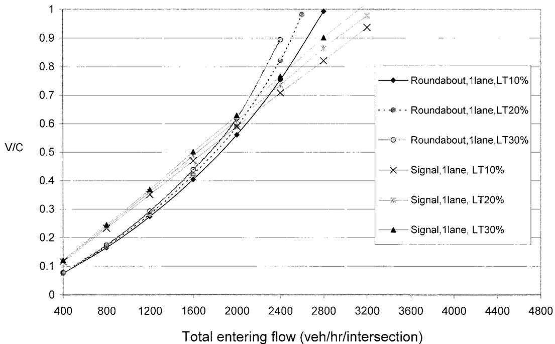
FIG. 5. Comparison of V/C for Roundabouts and Signalized Intersections (1-Lane Approaches, 4 Leg)
