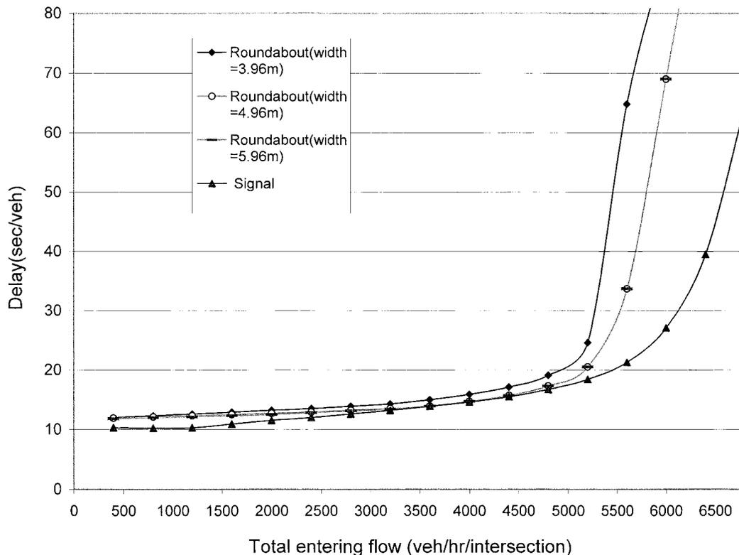
FIG. 3. Comparison of Delays under Various Intersection Types (3-Lane Approaches, 4 Leg, LT = 10%)
