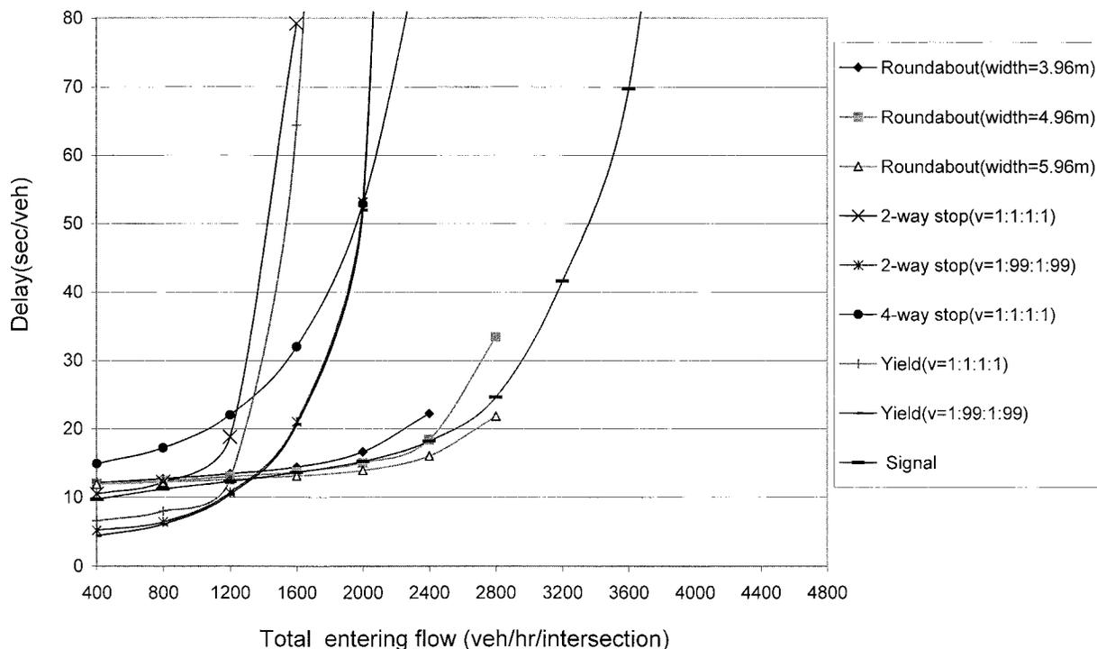
FIG. 1. Comparison of Delays under Various Intersection Types (1-Lane Approaches, 4 Leg, LT = 10%)
