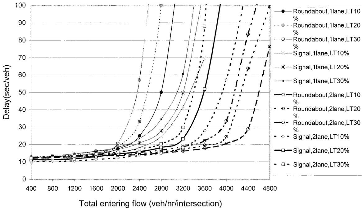
FIG. 4. Effect of Left-Turn Percentage on Delay for Roundabouts and Signalized Intersections
