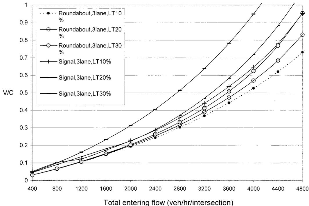
FIG. 7. Comparison of V/C for Roundabouts and Signalized Intersections (3-Lane Approaches, 4 Leg)
