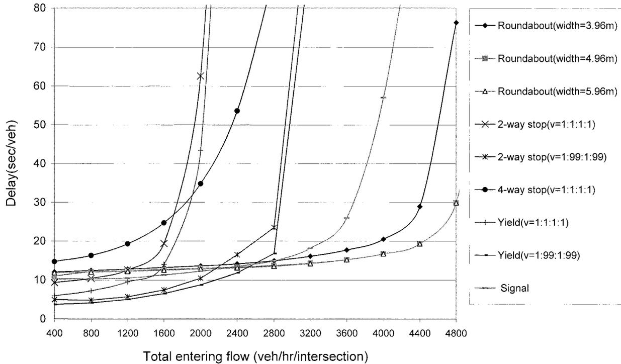
FIG. 2. Comparison of Delays under Various Intersection Types (2-Lane Approaches, 4 Leg, LT = 10%)
