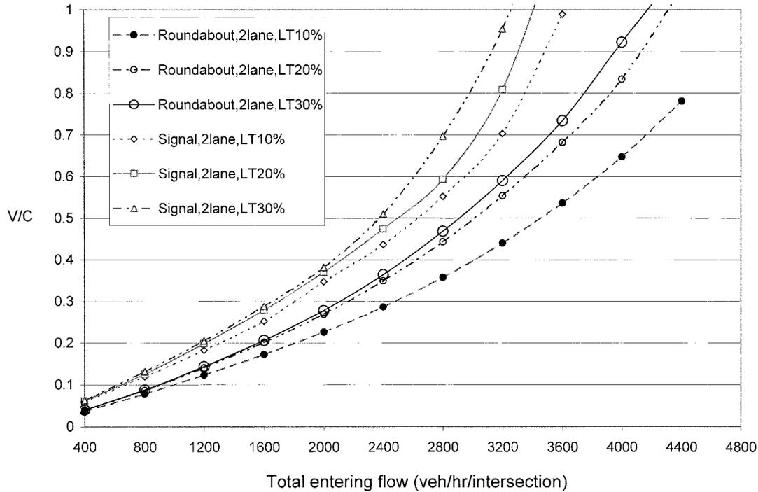
FIG. 6. Comparison of V/C for Roundabouts and Signalized Intersections (2-Lane Approaches, 4 Leg)
