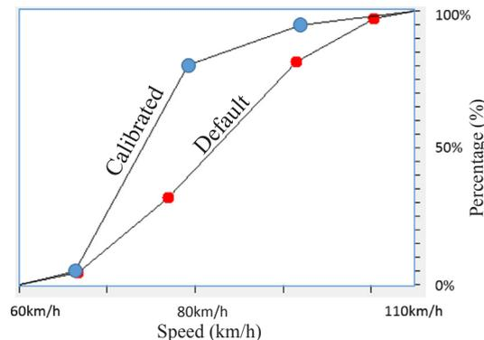
**Fig. 3.** Default vs. calibrated traffic speed distribution in VISSIM.
