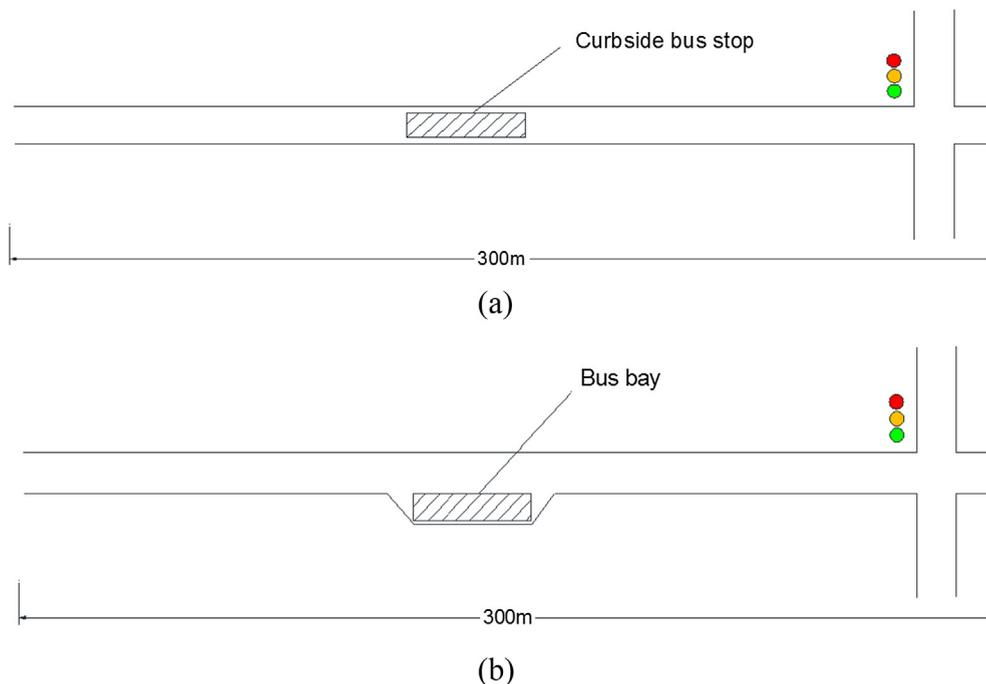
Fig. 2. Modelled road links with: (a) curbside bus stop and (b) bus bay.
