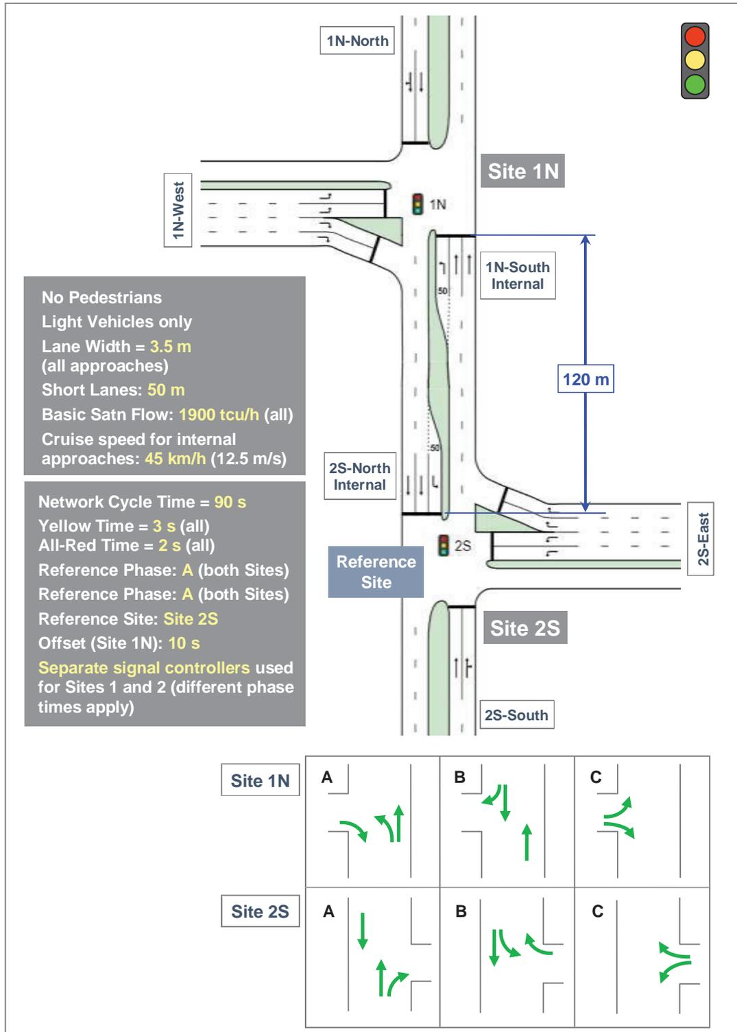
Figure 1 - Example: staggered-T intersection network (for both Scenarios (i) and (ii))
