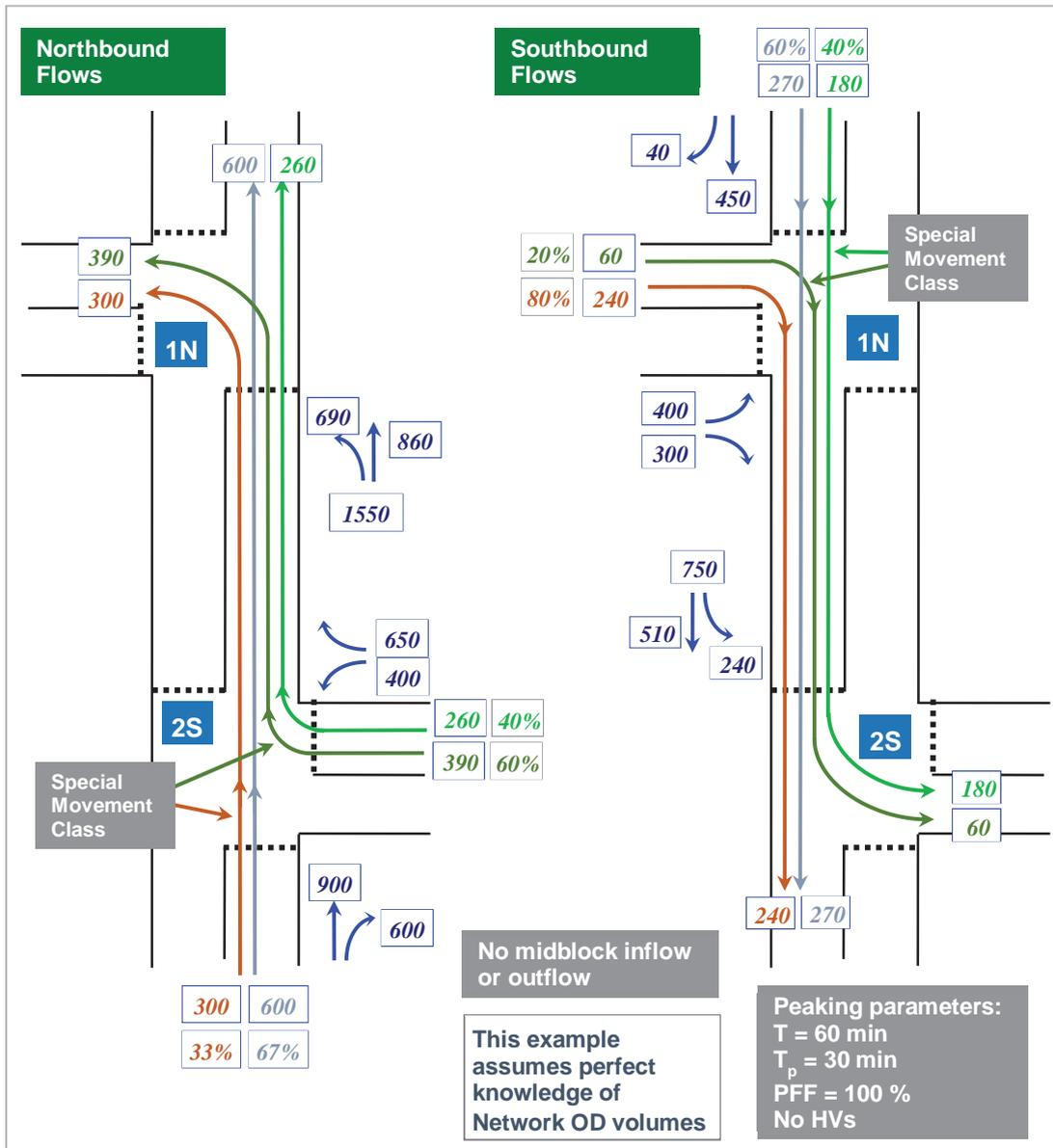
Figure 2 - Site and Network origin - destination (OD) flows for the example shown in Figure 1
