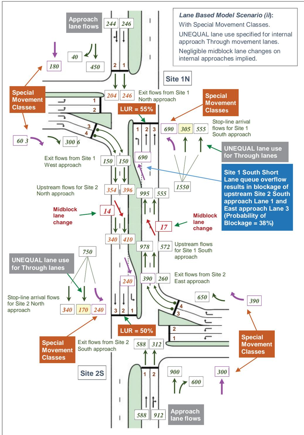
Figure 5 - Scenario (ii): WITH Special Movement Classes and UNEQUAL lane use for internal approach Through movement lanes for the example shown in Figures 1 and 2
