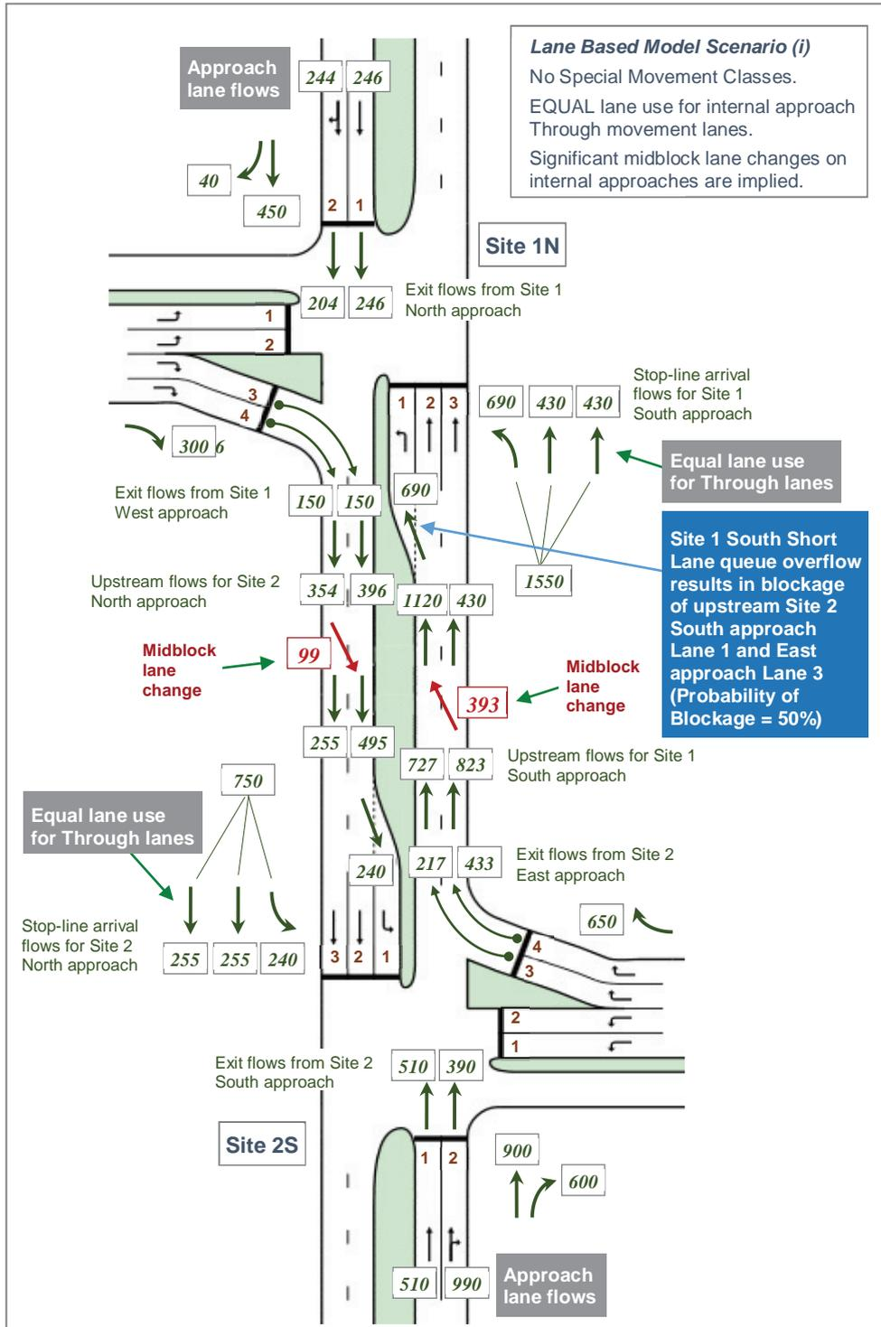
Figure 4 - Scenario (i): No Special Movement Classes and EQUAL lane use for internal approach Through movement lanes for the example shown in Figures 1 and 2
