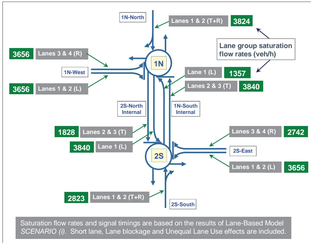
Figure 3 - Network specification and saturation flow rates for the Lane-Group Based Model for the example shown in Figures 1 and 2
