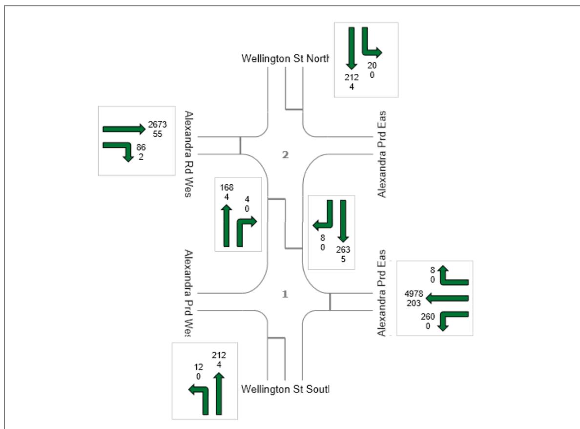
**Figure 4** Equivalent hourly flow rates (veh/h) of demand flows used for the analysis of the intersection of Wellington St and Alexandra Parade during 7.45 - 8.00 AM
