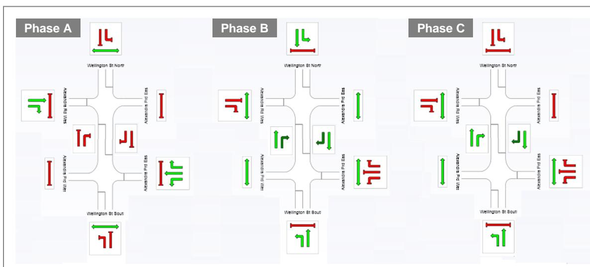
Figure 5 Signal phasing for the intersection of Wellington St and Alexandra Parade
