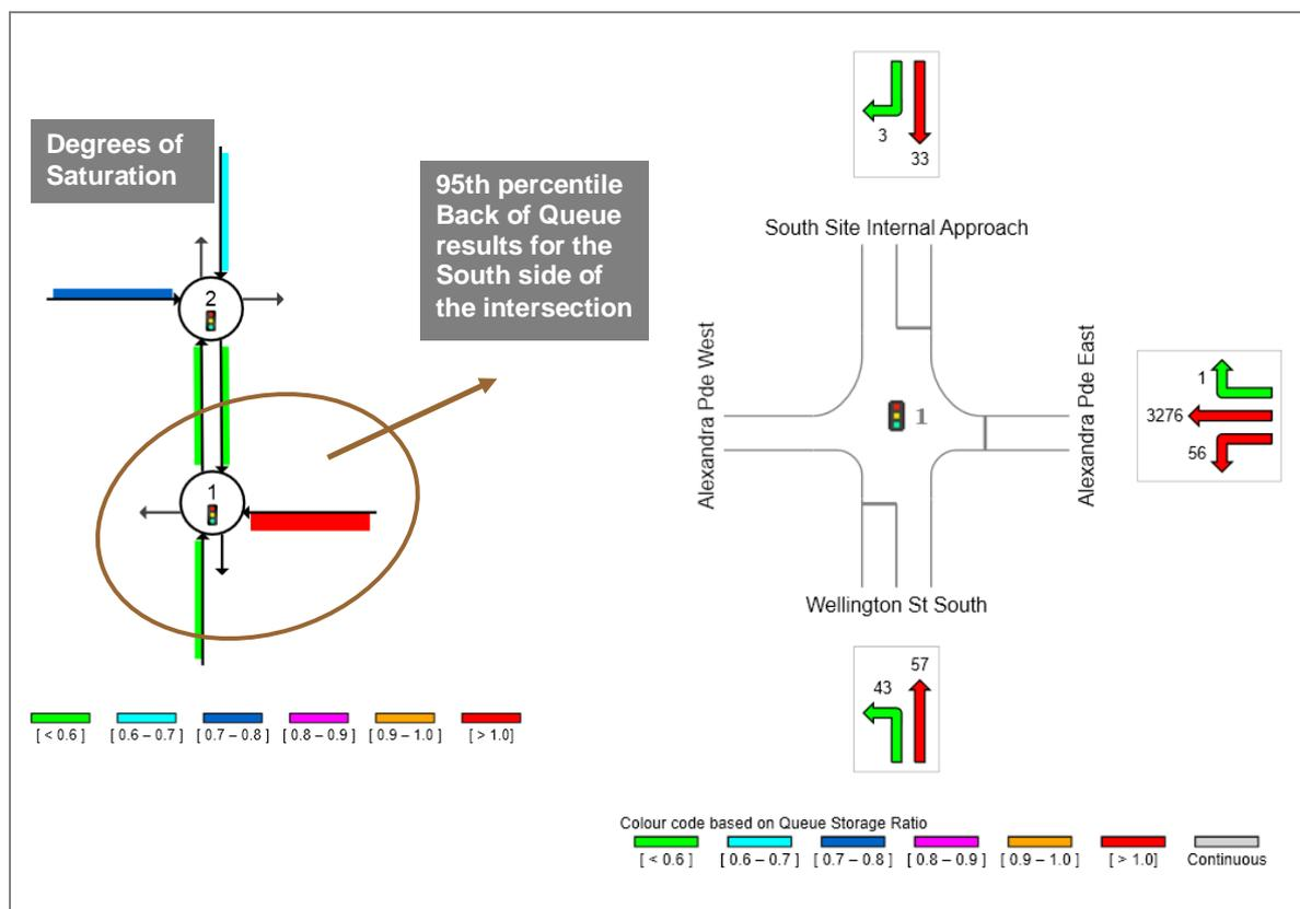
**Figure 7 SIDRA INTERSECTION displays for the Demand Model applied to the 7.45 - 8.00 AM peak period**
