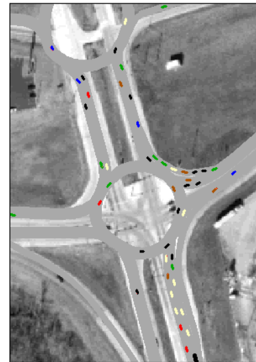
VISSIM simulation of a potential roundabout.
