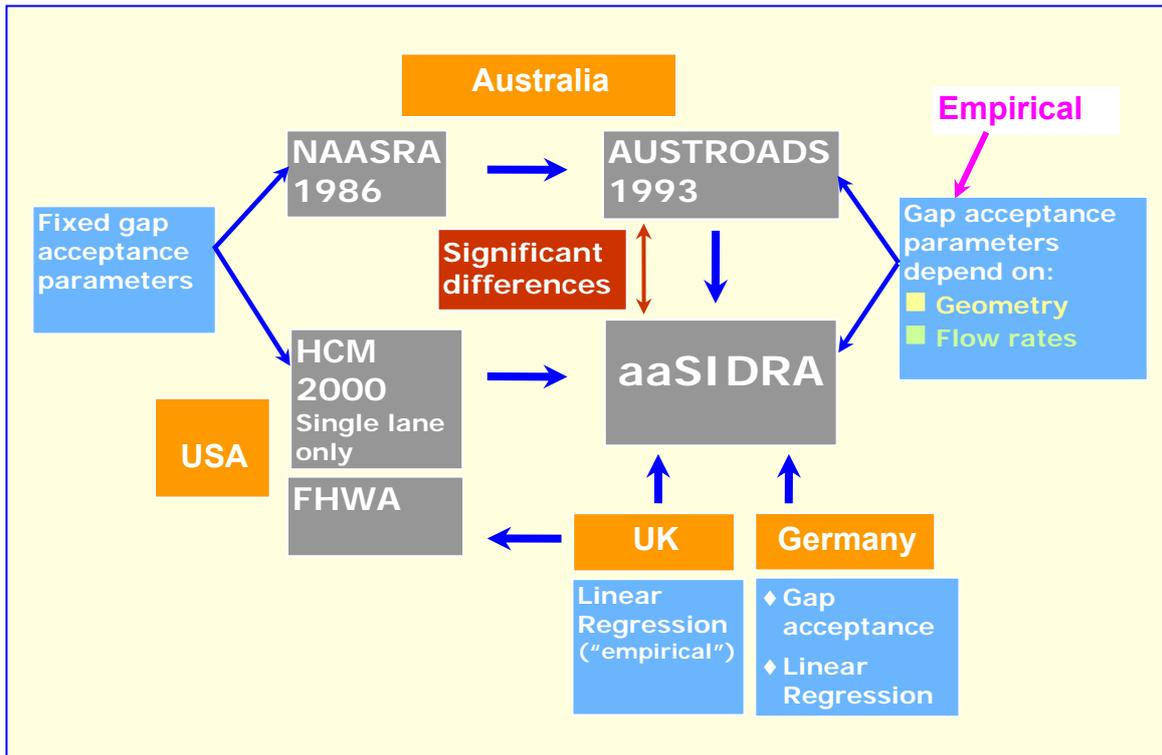
**Figure 1.1 - Relationships among roundabout analysis models related to the aaSIDRA model, or used in aaSIDRA as alternative models**
