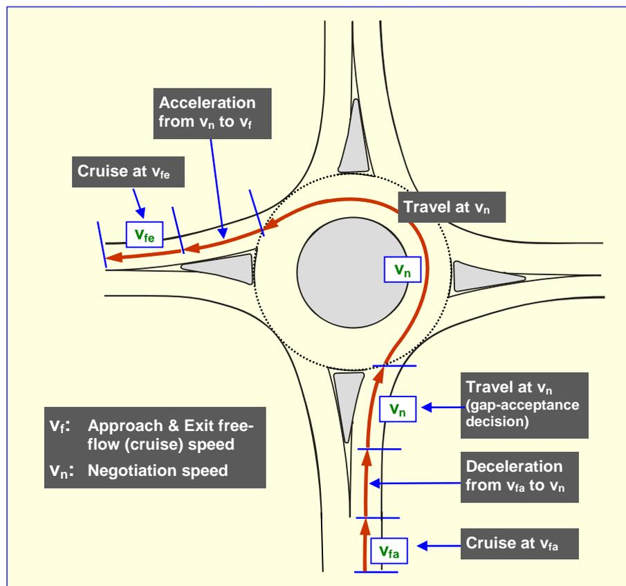
Figure 4 - Geometric delay parameters
