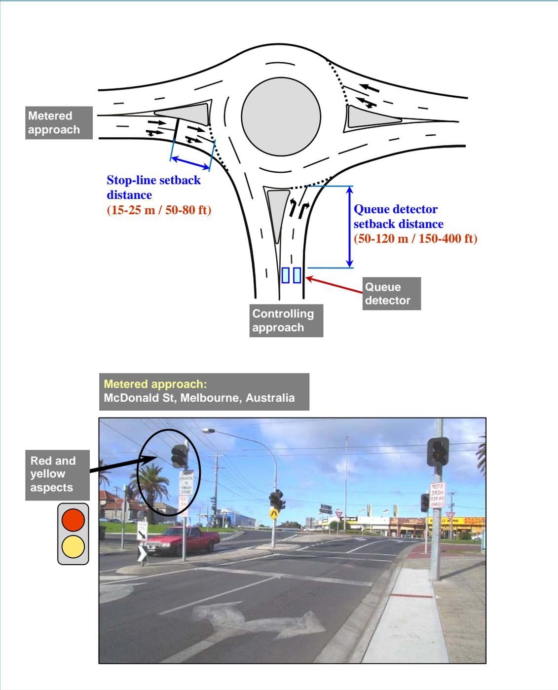
Figure 5 - Roundabout metering signals
