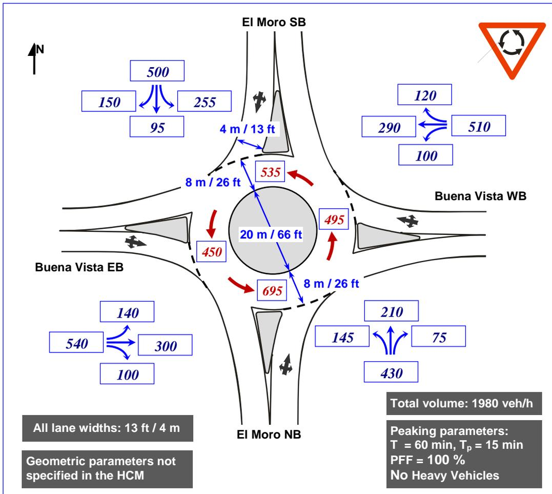
Figure 1 - Example 1: single-lane four-way roundabout given in HCM 2000, Chapter 17 (23)
