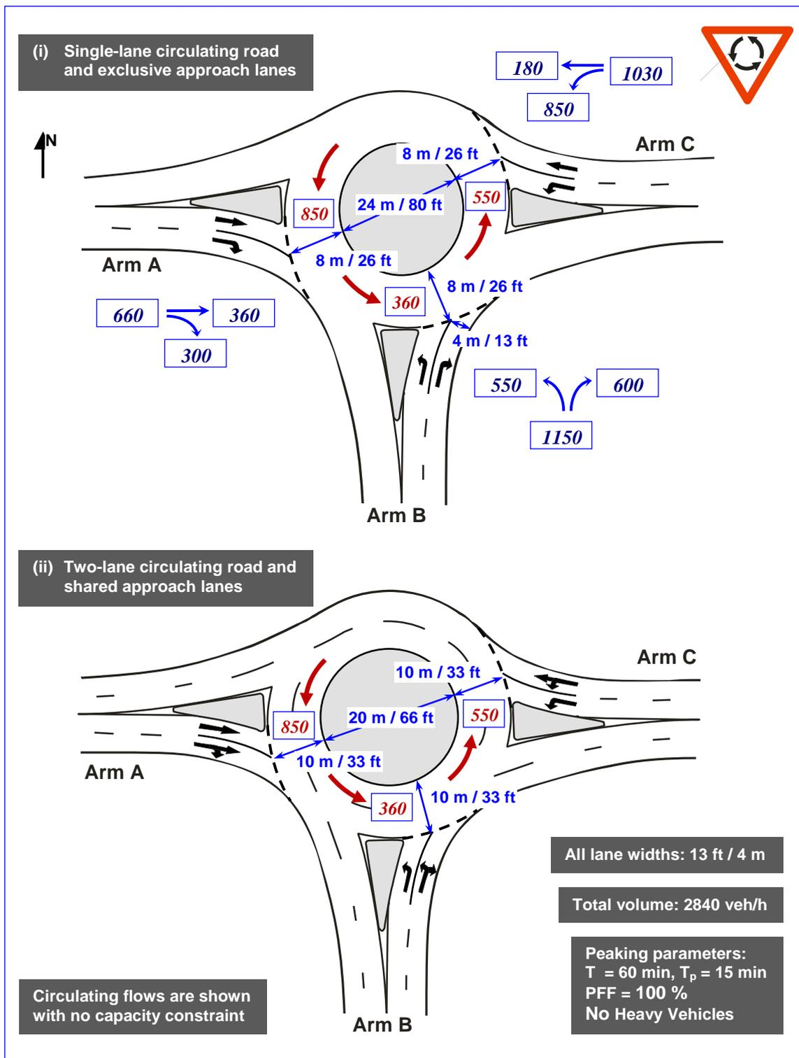
Figure 2 - Example 2: two cases of T-intersection roundabout lane arrangements based on an example given by Chard (24, 25)
