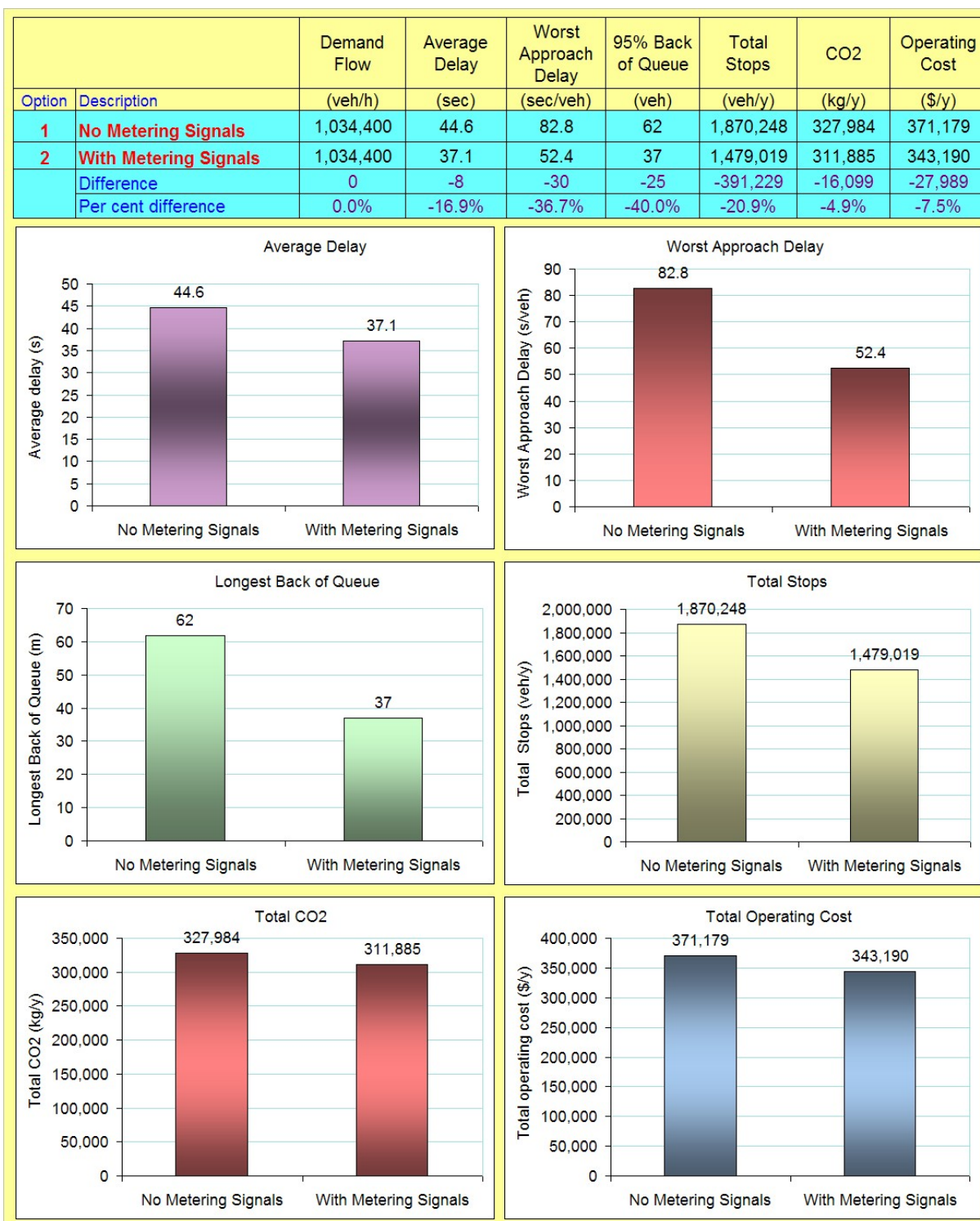
Figure 11 - Benefits from metering signals for the Mickleham Rd and Broadmeadows Rd Roundabout
