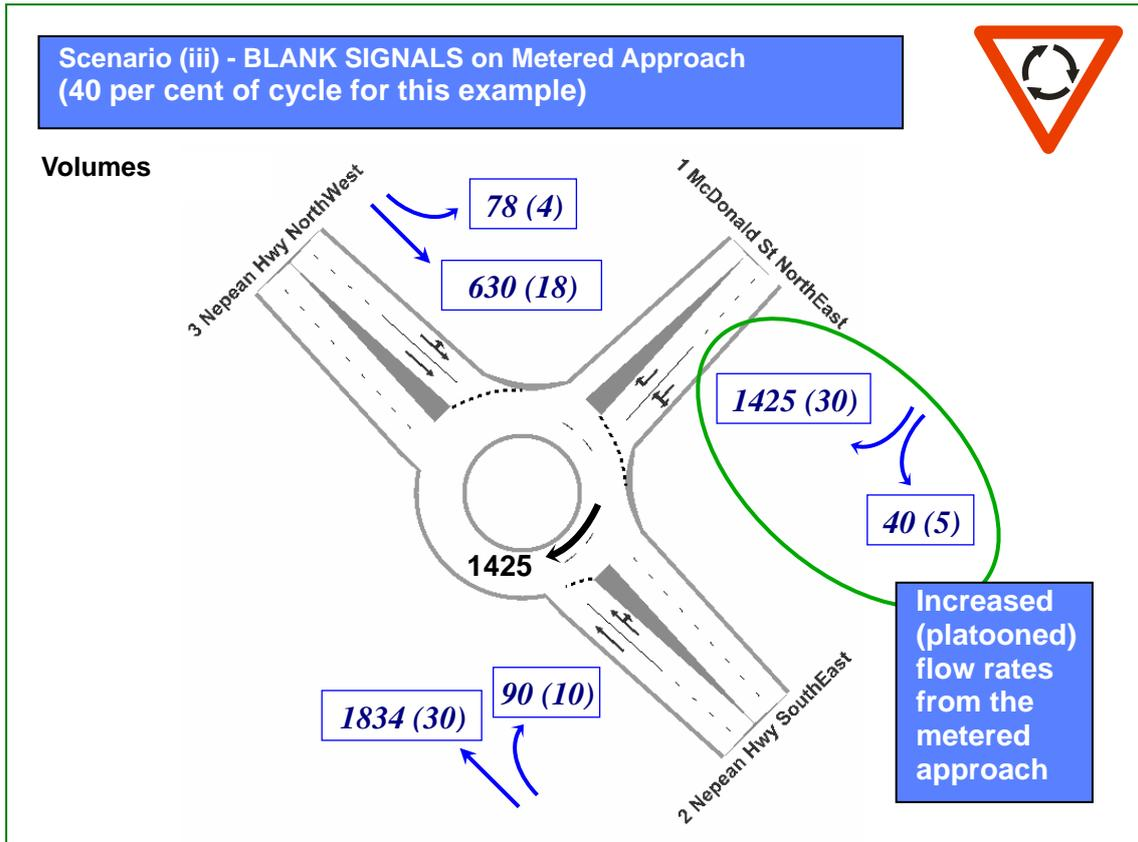
Figure 6: Roundabout operating with BLANK signals on the metered approach (McDonald St) - platooned flow rate entering from the metered approach
