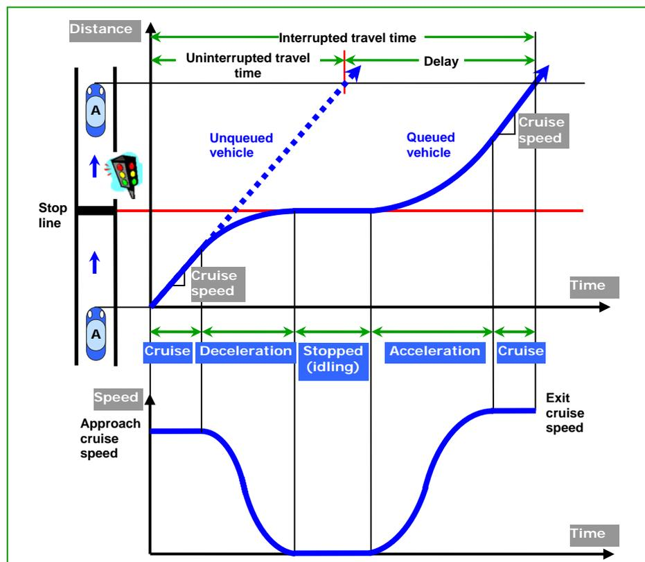
Figure 1: Drive cycle during a stop at traffic signals (example)
