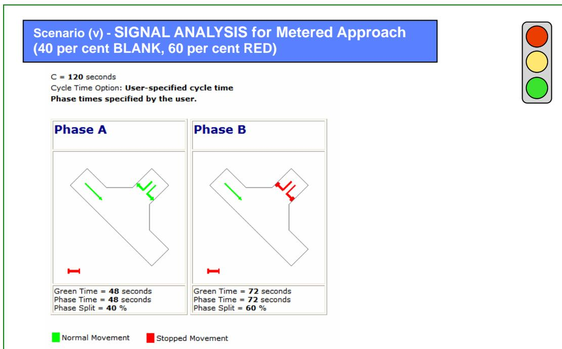
Figure 7: Metering signal timing analysis for the Nepean Highway - McDonald Street roundabout
