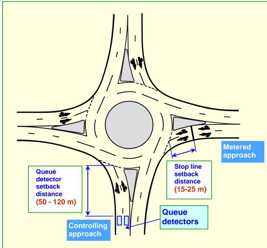
Figure 2: Typical arrangements for roundabout metering signals
