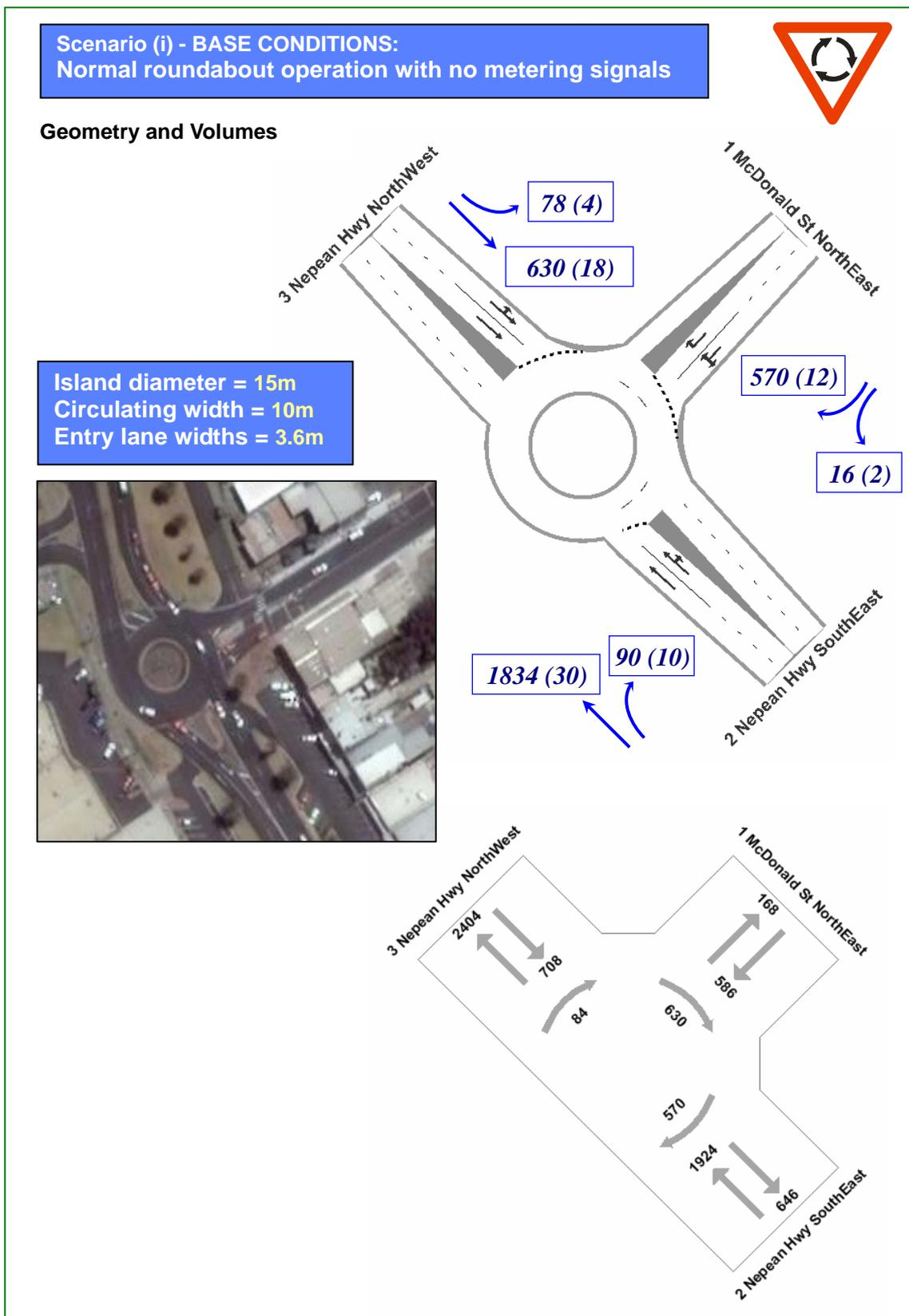
Figure 4: Roundabout operating without metering signals (base condition)
