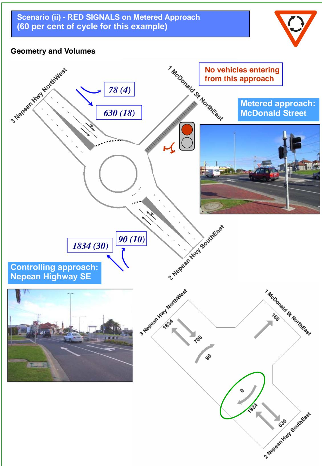
**Figure 5: Roundabout operating with RED metering signals on the metered approach (McDonald St)**
